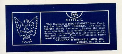
By the improved method we use in manufacturing these hammers as explained on our label shown above, EVERY HAMMER IS EXACTLY THE SAME IN SHAPE AS WELL AS TEMPER.
