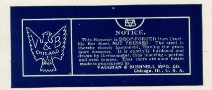
By the improved method we use in manufacturing these hammers as explained on our label shown above, EVERY HAMMER IS EXACTLY THE SAME IN SHAPE AS WELL AS TEMPER.
